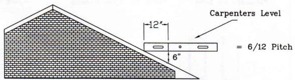
Place the level on the roof as shown(level). Measure out 12" from the BOTTOM corner of the level. From that point, measure straight down to the roof surface. That distance over 12 is the roof pitch.
